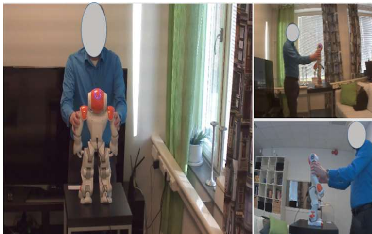
Figure 2. Experimental set-up where the participant interacts with the NAO in the Usability Lab. The participant interacts with the NAO by touching left and right arms to convey a particular emotion. Camera shots are configured using the ELAN annotation tool: https://tla.mpi.nl/tools/tla-tools/elan/ .
