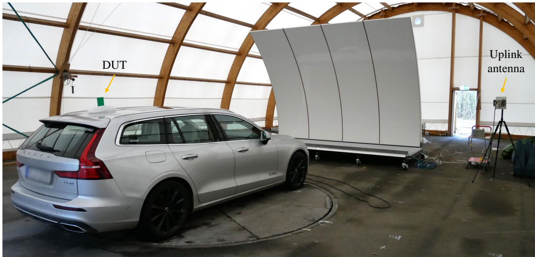
Figure 5.7: Picture of the active measurement setup for vehicles, using the sub-6 GHz system [B].
