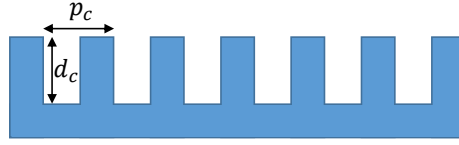
Figure 3.2: Corrugated surface with the corrugation depth d_c and periodicity p_c .
