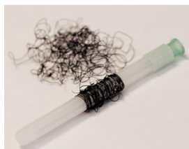
Figure 2. Photograph of melt-spun PEDOT:Nafion fibers, wrapped around a 5 mm wide syringe cover.
