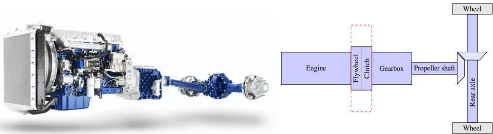
Figure 2.1: Truck powertrain, source: AB Volvo (left) and schematic picture of powertrain (right)
