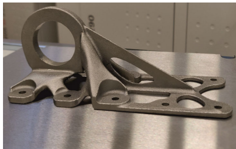
Figure 3: A topologically optimized bracket for an aerospace application produced at Chalmers using a design developed with the aid of Simufact Additive simulations.
