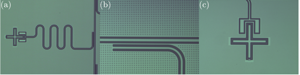
Figure 2.2: (a) A coplanar waveguide resonator coupled to a transmon qubit. (b) Inductive resonator to transmission line coupling. Visible is also the flux-trapping holes. (c) Resonator to qubit coupling. The ground plane extends all around the qubit, ensuring a good microwave environment.
