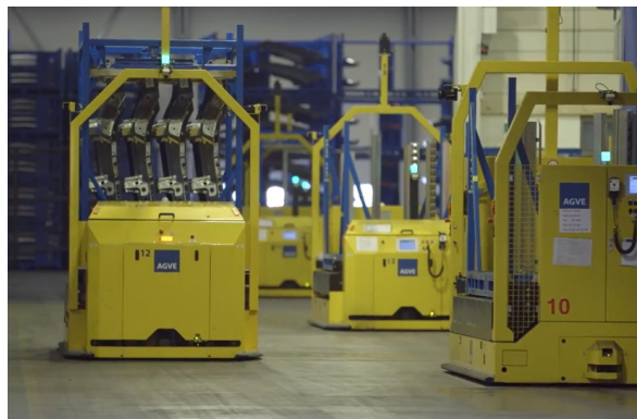
Figure 5.1: AGVs in the Volvo Cars plant. The left vehicle carries a rack loaded with sheet metal parts.
