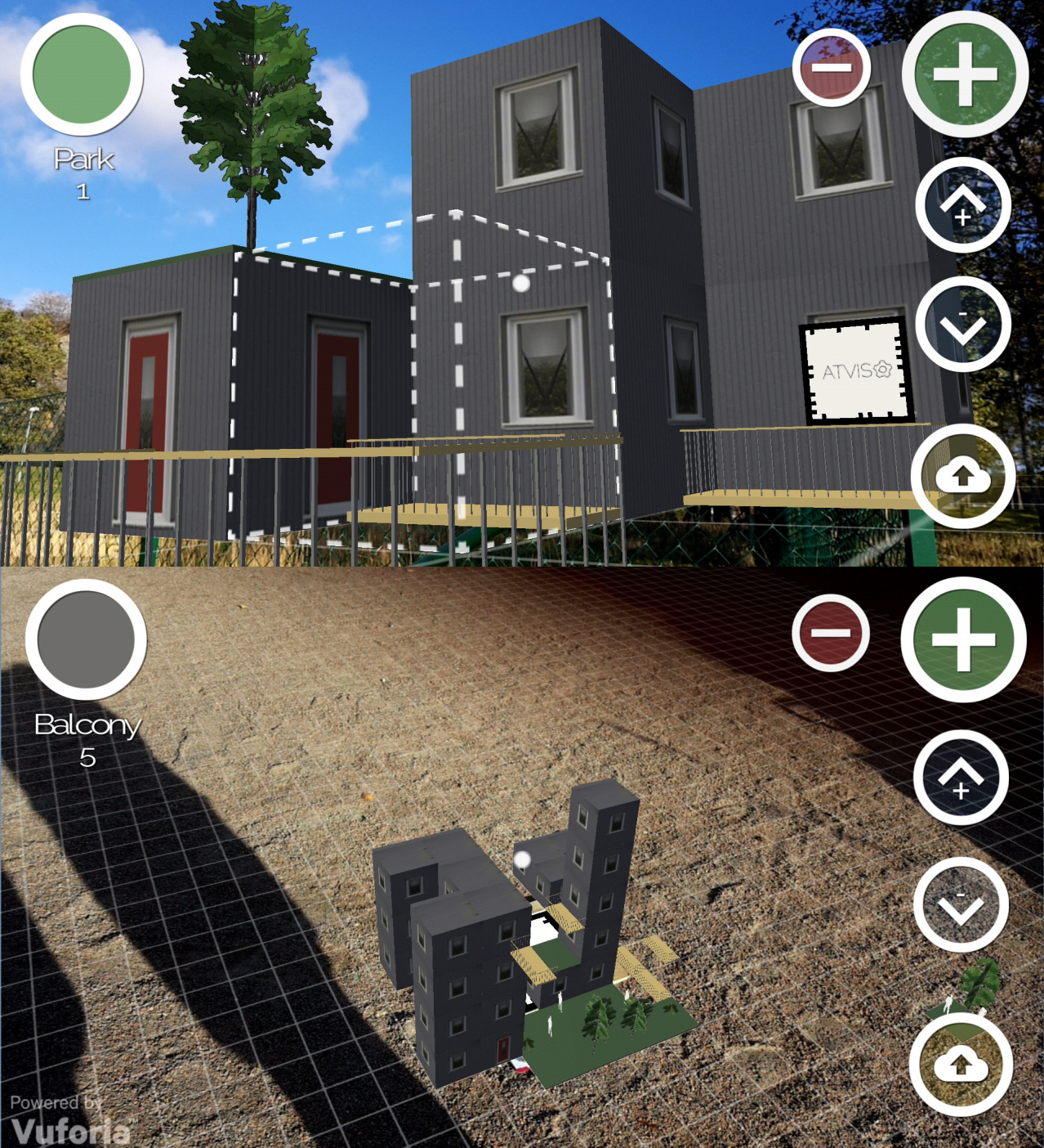
Screenshots of Urban CoBuilder in use: Top image shows its use as a 1:1 scale design app and the bottom image shows a tabletop version scaled-down model. The images were taken during the student workshop at Hammarkullen, 2018.
