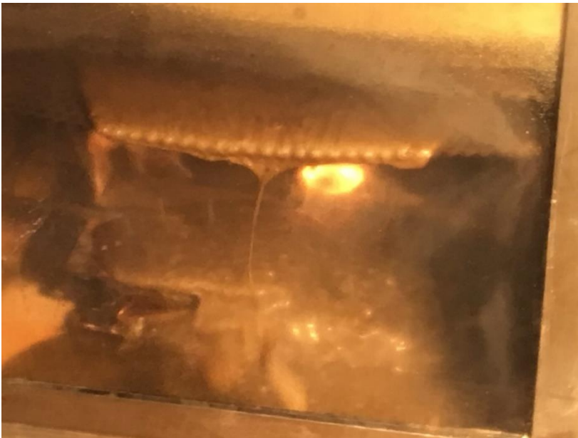
Figure 19 The spread of the AVD agent over the perforated horizontal steel sheet plates, prior full fire extinguishment.
