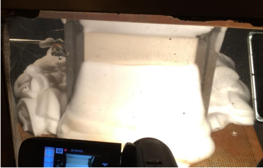
Figure 18 The fill-up of “dry” CAFS foam inside the simulated battery module in Test 37.
