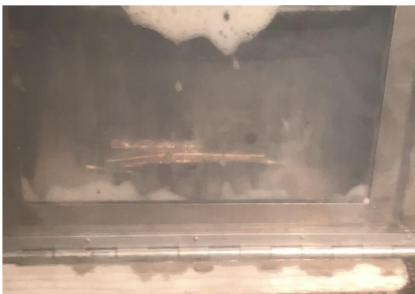
Figure 17 The incomplete fill-up of “dry” CAFS foam inside the simulated battery module in Test 36.
