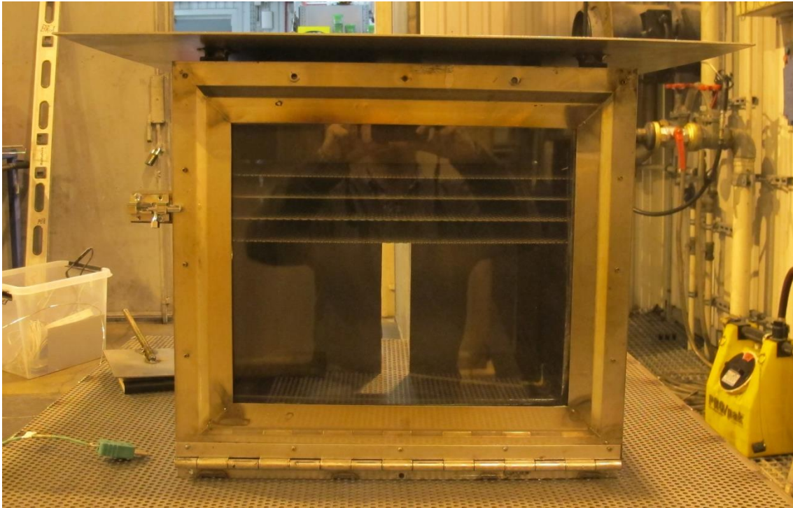
Figure 2 The simulated battery module was fabricated from metal sheets with a frame size of 400 mm by 400 mm by 400 mm (height). One side consists of a fire rated glass window to facilitate visual observations and video recordings.
