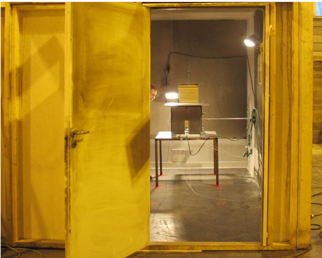
Figure 4 The simulated battery module was positioned on a table inside the test compartment.
