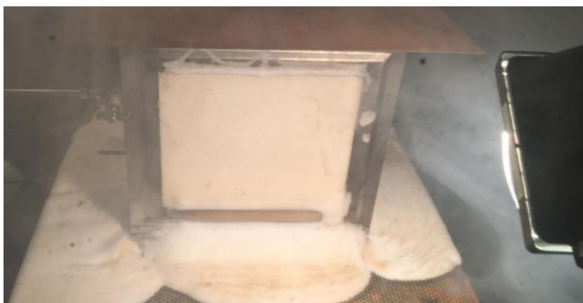
Figure 16 The fill-up of “wet” CAFS foam inside the simulated battery module foam in Test 35.
