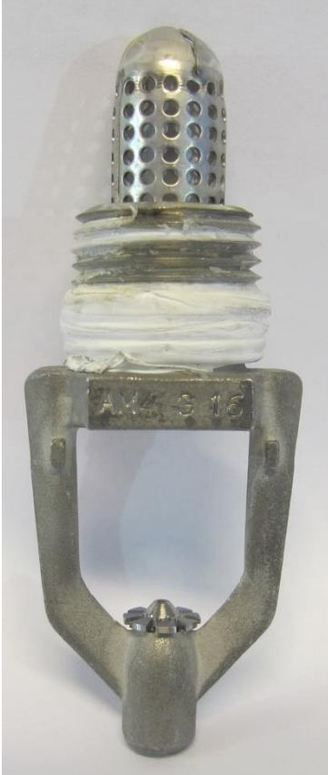
Figure 8 The pendent open (non-automatic) low-pressure single-orifice water mist nozzle used in the total compartment system tests.
