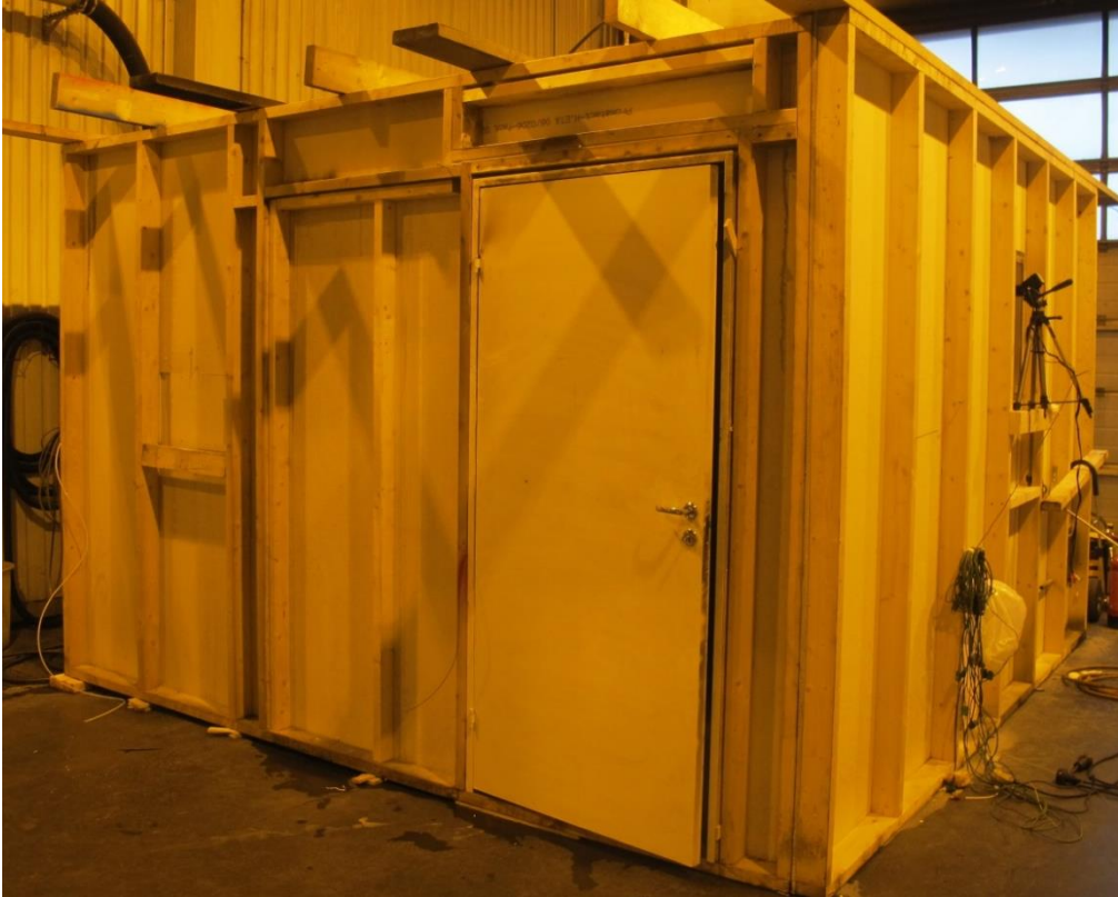
Figure 3 The fire test compartment used in the tests. The compartment was sized 3.66 m by 3.66 m and had a regular doorway opening at one of the walls. The video camera providing a room overview is seen to the right.
