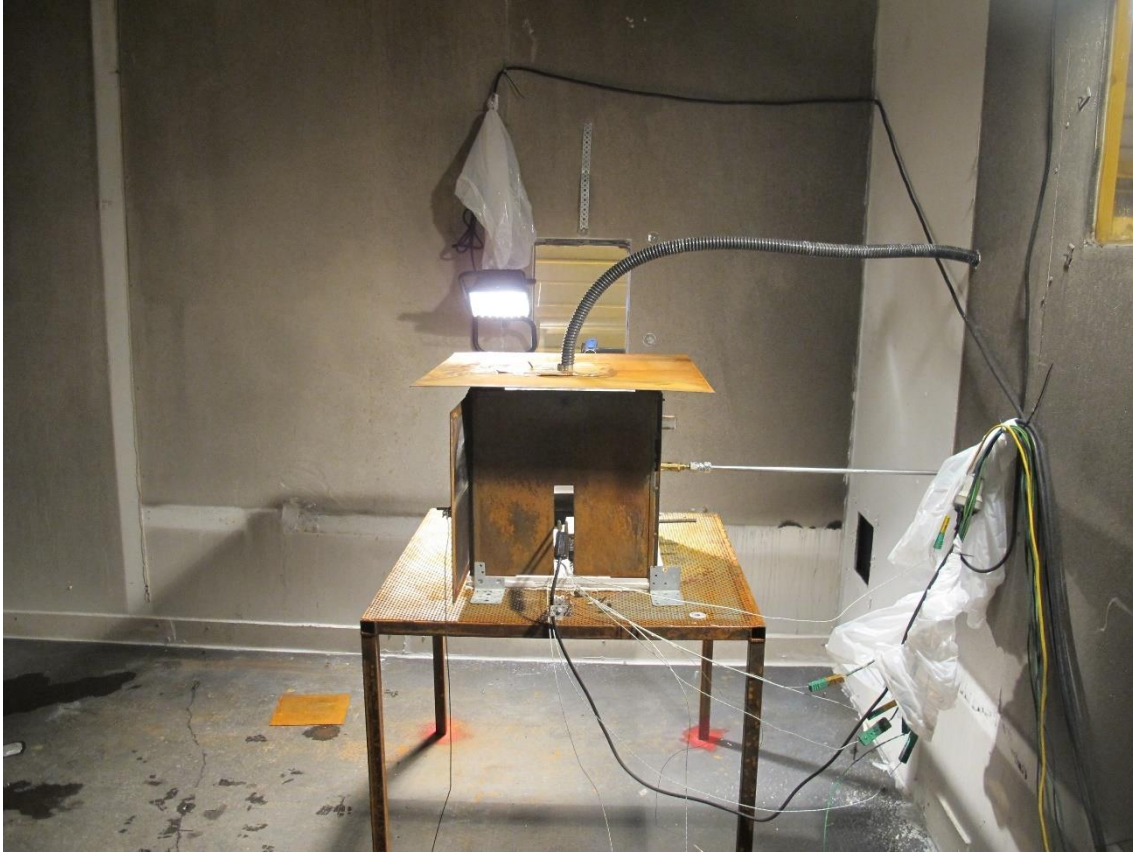
Figure 12 The connection of the nitrogen gas hose line to the top of the simulated battery module.
