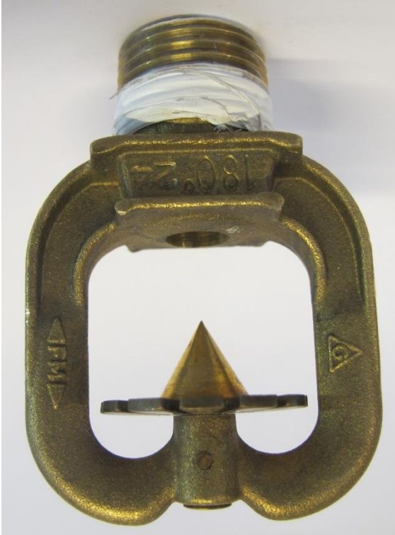
Figure 7 The pendent open (non-automatic) medium velocity water spray nozzle used in the total compartment system tests.
