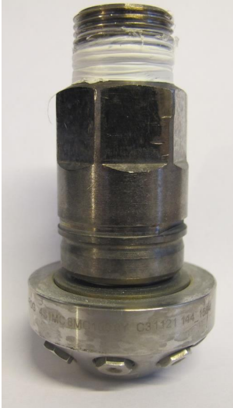
Figure 9 The open (non-automatic) high-pressure water mist nozzle used in the total compartment system tests.
