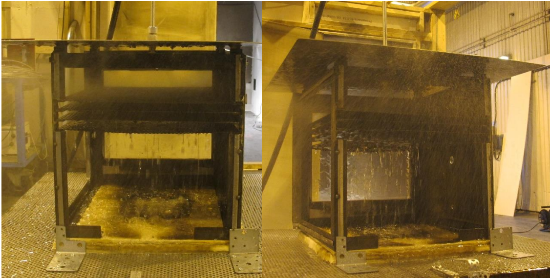
Figure 11 Distribution of water inside the simulated battery module when discharging 5.0 liter/minute (left) and 7.1 liter/minute (right), depicted from the backside of the simulated battery module, with the back wall removed.
