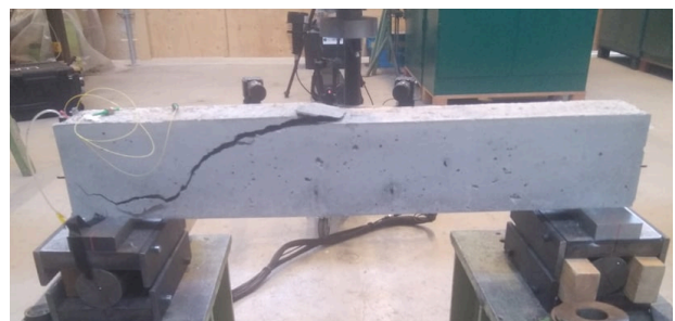
Figure 3. Tested beam after failure.
