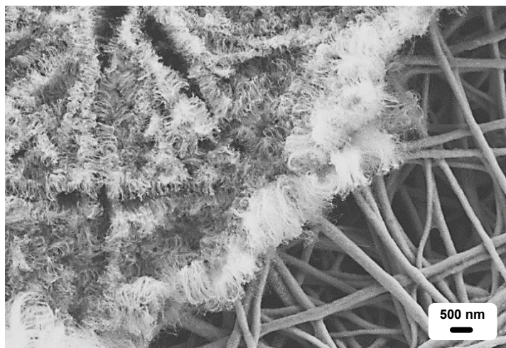
Figure 3.6 SEM image of the border between pure CNF and CVD grown CNT on CNF
