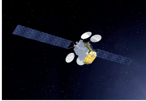
Figure 1.3: A GEO satellite with four array-fed reflectors (Eutelsat/Thales Alenia Space Broadband for Africa High Throughput Satellite) [11].
