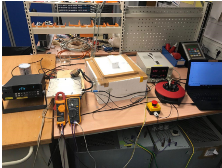
Figure 3.6: Laboratory set-up for the calorimetric measurements.
