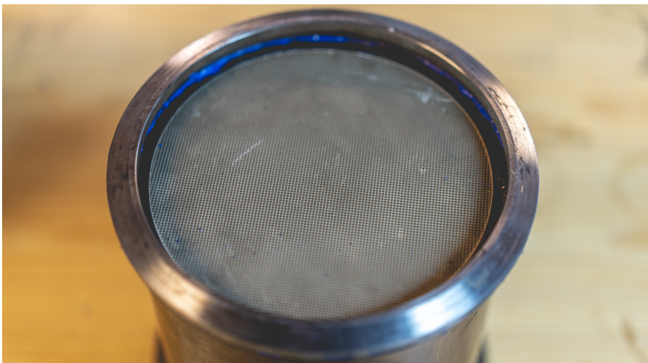
Figure 2.2: Photograph of a 400 CPSI ceramic monolith placed inside a metal canning.
