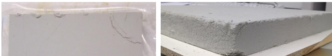
Figure 13: Obvious damage to the samples before measurement. Left: source: CRMgroup; right: source: Deutsches Zentrum für Luft- und Raumfahrt.
