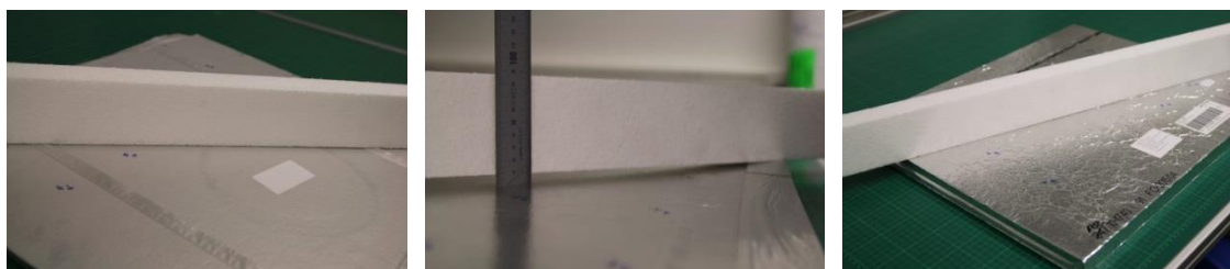
Figure 118: Left: specimen A, 10mm, flat; middle: specimen B, 10mm, curved; right: specimen C, 30mm, flat. (FIW München)
