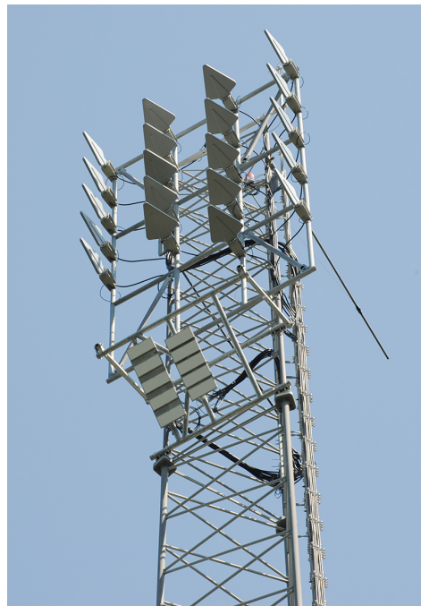
Figure 5. Photo of the antenna array at the top of the BorealScat tower. The small array at the bottom is for C-band only. The calibration procedure in this article focuses on the array at the top, which was designed for P to L-band, but is also valid for observations using the C-band array.
