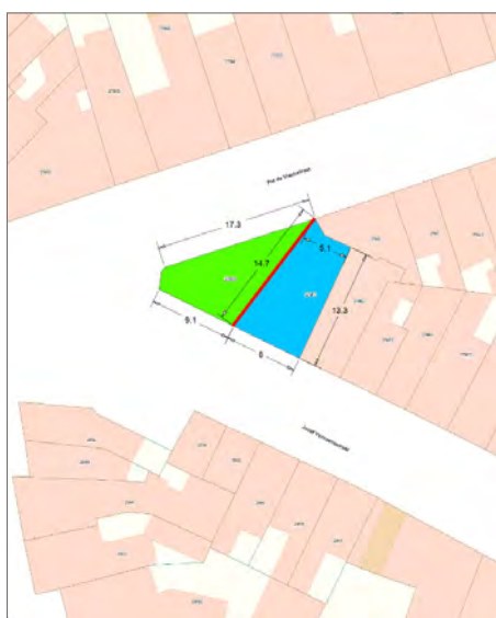
Figure 2.18: Excerpt from the design brief: site plan with suggestion for a zone for a private house (blue), a zone for a public square (green), and a red non-dimensional line separating both. In the design, the negotiation of that line and its dimensions became a leitmotiv.
