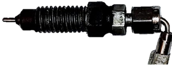
Figure 7. A modified bleeding screw for measuring brake fluid temperature.
