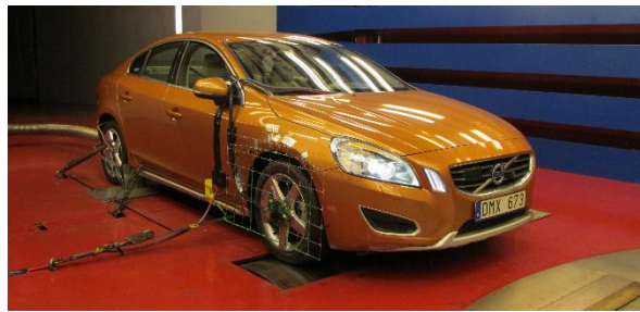
Figure 6. Test object during the wind tunnel braking investigation.
