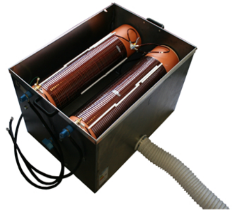
Fig. 7: Three-phase RL load, aircoil with forced air cooling.
