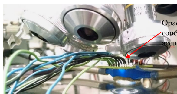
Figure 7. Measurement set-up: (a) generating soot for reproducible distribution; (b) window in the 3D-printed housing; (c) window under inspection during exposure.
