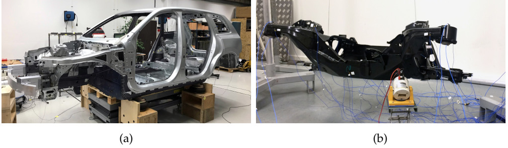
Figure 2.1: Experimental set-up of a BIW on air springs in (a) and rear subframe hanging in lines in (b).
