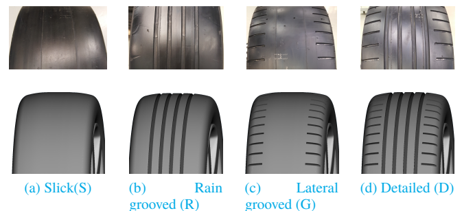
Figure 1: Investigated tyre sets: physical (top) and virtual (bottom).
