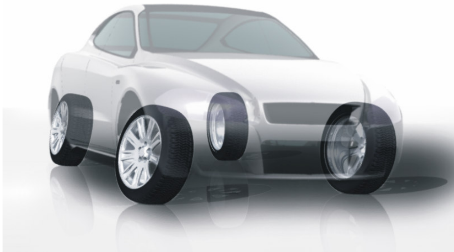
Figure 3. An illustration of a cornering manoeuvre of a vehicle with an ACM chassis (the vehicle is turning left at high speed). Negative camber angles of outer wheels and individual steering of the wheels combined can be used to obtain high lateral acceleration. Note the vertical force intervention lowering the left side of the vehicle body and tilting it in toward the curve to achieve desired comfort (18).
