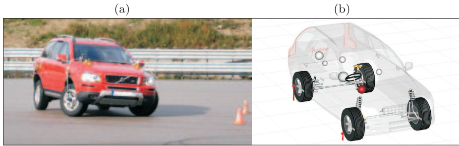
Figure 6.1: (a) Handling measurements carried out with an instrumented vehicle. (b) vehicle model developed in Dymola.
