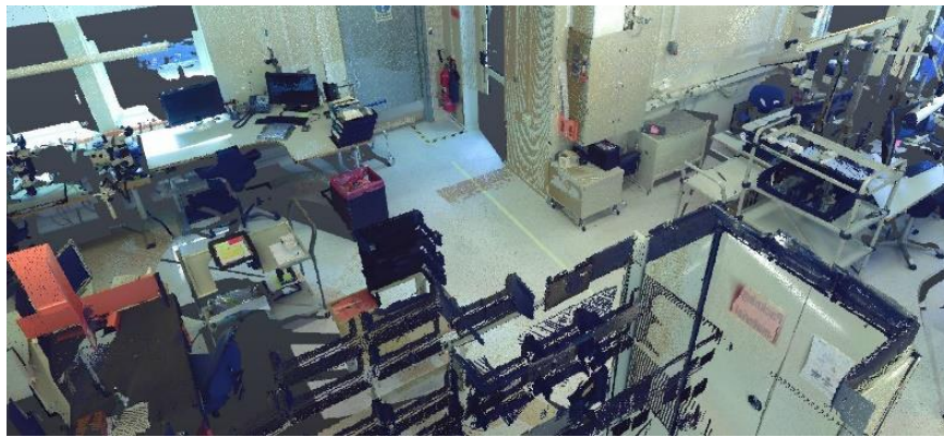
Figure 12: Visualisation of the spatial data gathered via 3D laser scanning.
