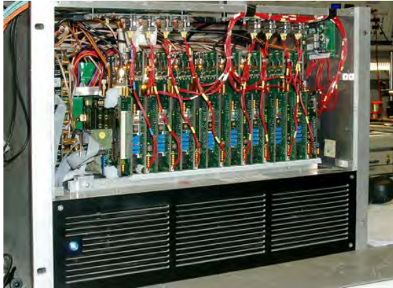
Fig. 1: DBBC3 VGOS model: 8 IFs with 8 groups of ADB3 samplers and CORE3 processing boards. This unit can deliver 128 Gbps with 2-bit samples (output limit is 512 Gbps).
