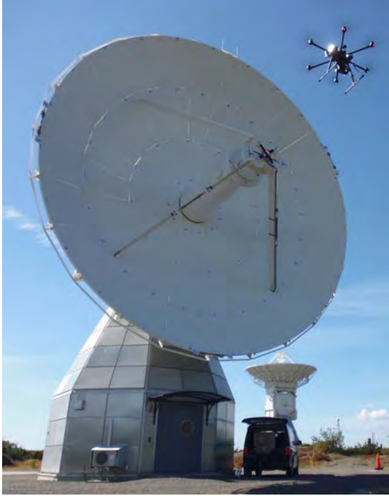
Fig. 2: The VGOS radio telescope ONSA13NE equipped with several coded markers, scale-bars and coordinate cross during the UAS-based photogrammetric survey of the main reflector surface.
