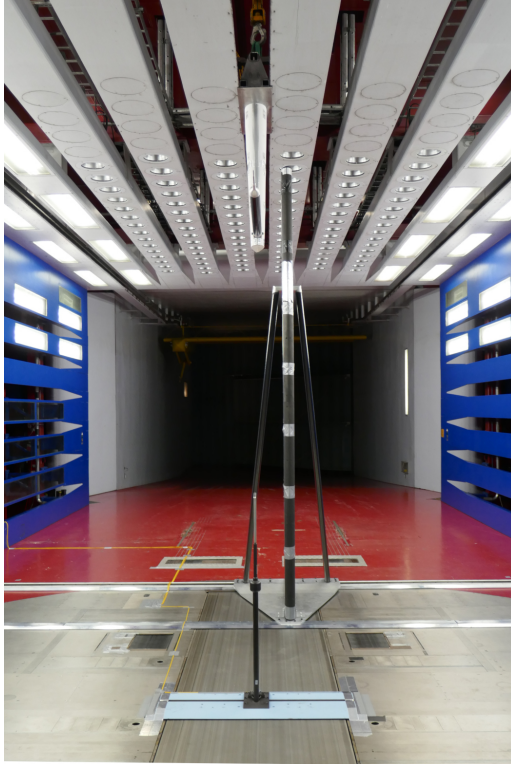
Figure 3.8: The interference measurement setup measuring static pressure in front of the FMR at z = 1.2 m and z = 3.1 m.
