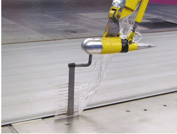
Figure 3.2: Boundary layer rake mounted on the traversing gear.
