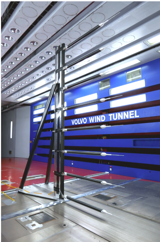
Figure 3.4: The new Flow Measurement Rig (FMR) mounted at the turntable center.
