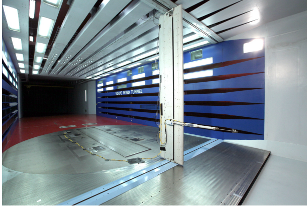
Figure 3.3: The old commissioning strut mounted at the upstream end of the test section.
