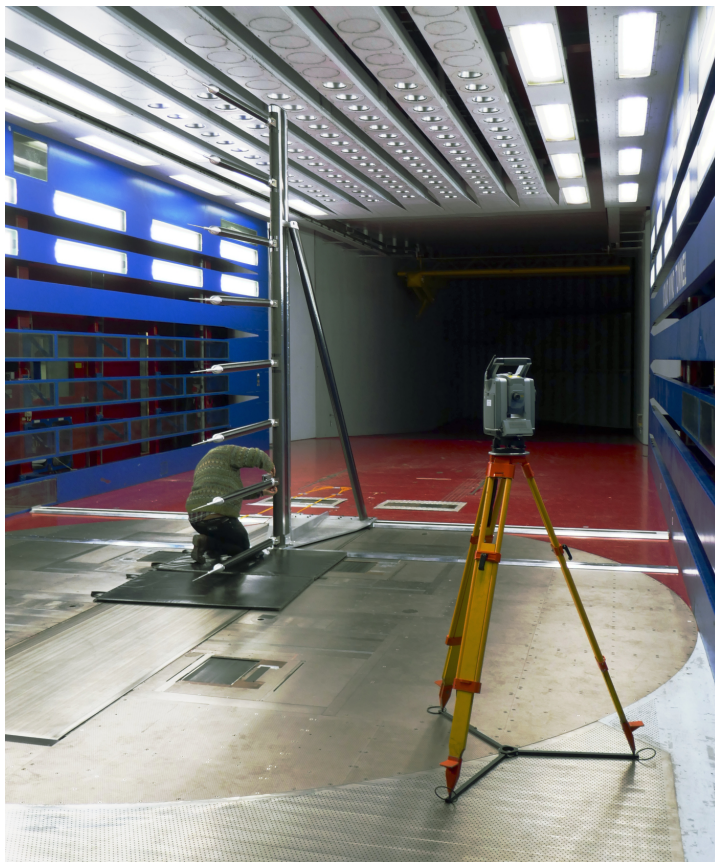
Figure 3.6: The total station used to measure the angles of the probe arms.
