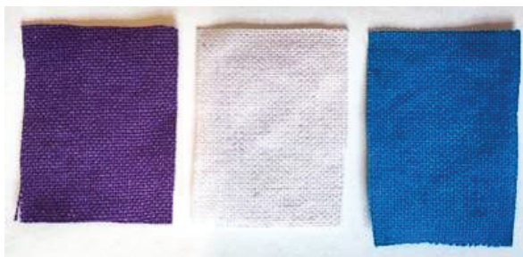
Figure 29. Reversible adsorption of nanoparticles of pigment on cationised cotton fabric, coloured with pigment PV23 ( left ), de-coloured from pigment PV23 ( middle ), recoloured with pigment HB 15:3 ( right ).
