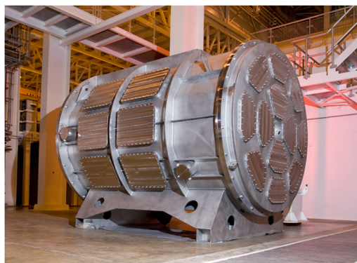
FIG. 6. The “as-delivered” Polaris sample tank. Photograph: STFC.
