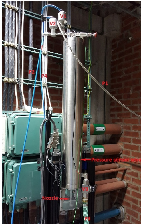
Figure 2 Photo of the continuous flow rig.
