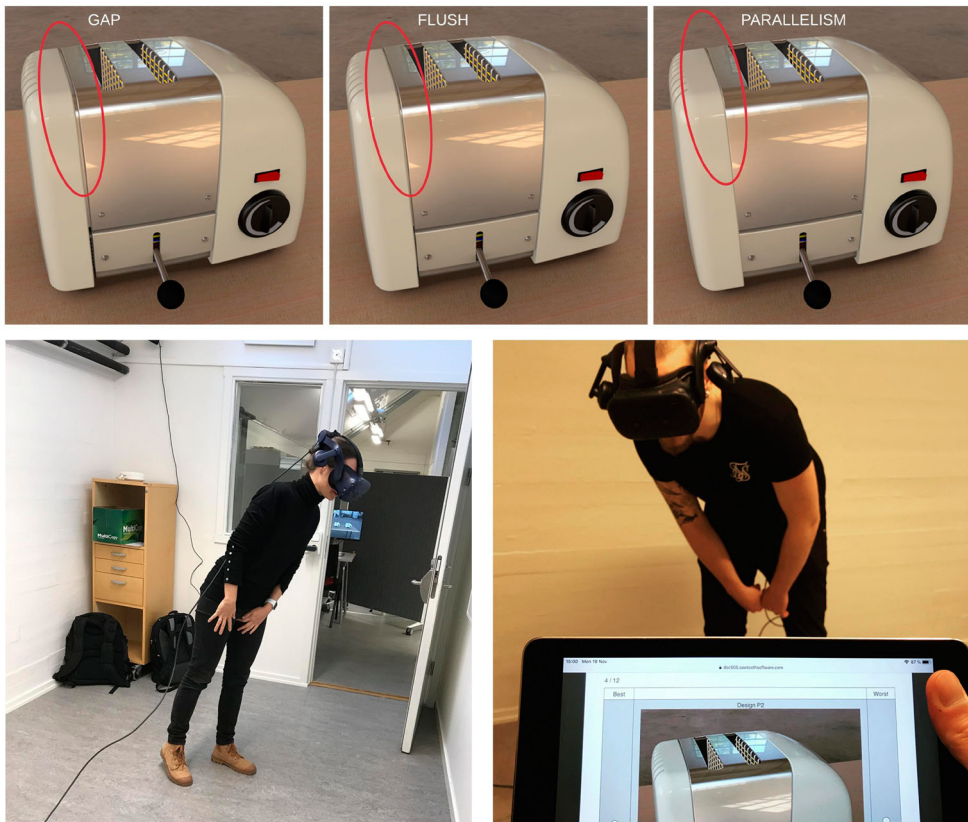
Figure 9. Fully immersive head-mounted display system exercise for evaluation of a bread toaster split-lines.
