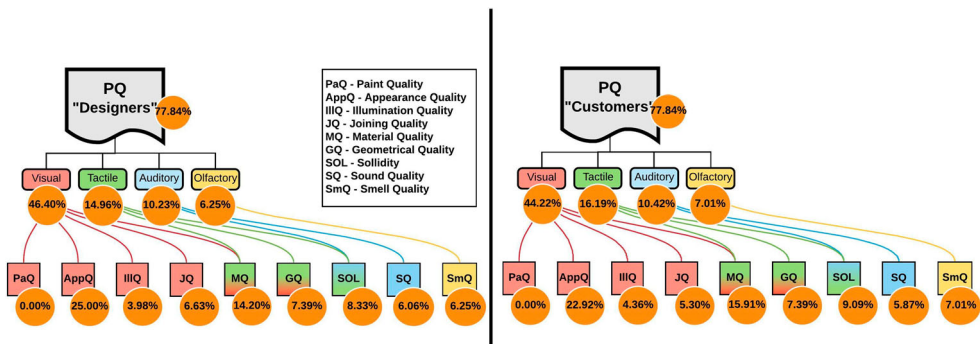
Figure 7. Perceived quality attributes importance ranking values for relevant PQF areas regarding a ‘generic’ SUV intended for the EU premium market segment for both teams.
