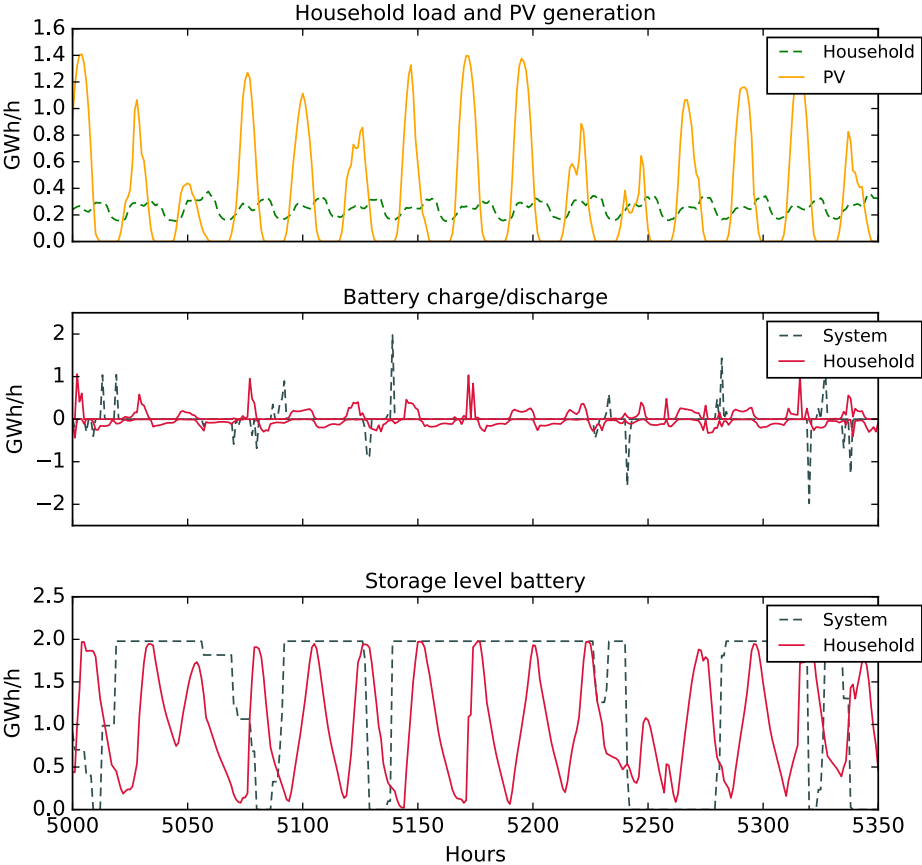
Figure 4: Load and PV generation profiles in the prosumer households. Shown are the charge (on the positive y-axis) and discharge (negative y-axis) patterns and storage levels of the batteries from the system perspective and from the prosumer household perspective. The data are for two modeled summer weeks, shown as the aggregate for the southernmost market region in Sweden. [adapted from Paper I].
