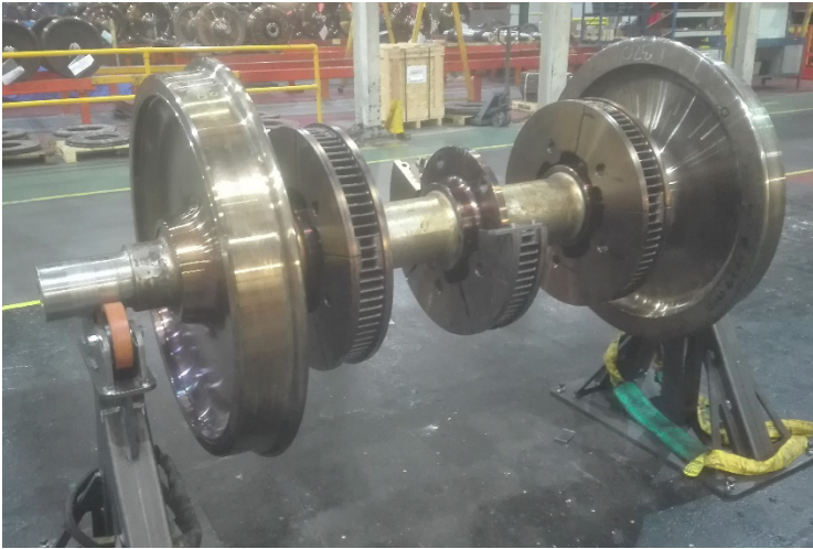
Figure 2 Wheelset equipped with segmented brake discs (only partially mounted segments).
