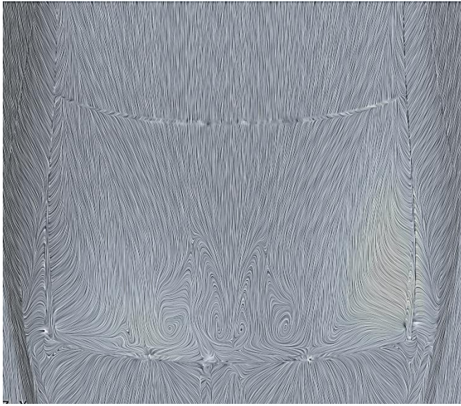
Figure 10: Limiting streamline pattern calculated in CFD for 30% Volvo S60 with the overhead strut
