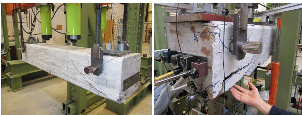
Fig. 4 Pilot tests with improved strengthening method at the suspension holes. Left: specimen without initial damage, after structural testing. Right: specimen with initial corrosion damage including cover spalling, upon failure.
