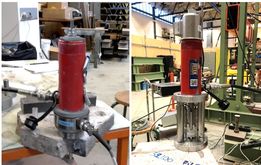
Fig. 11 Pull-out test setup, (left) in pilot test and (right) with developed rig.
