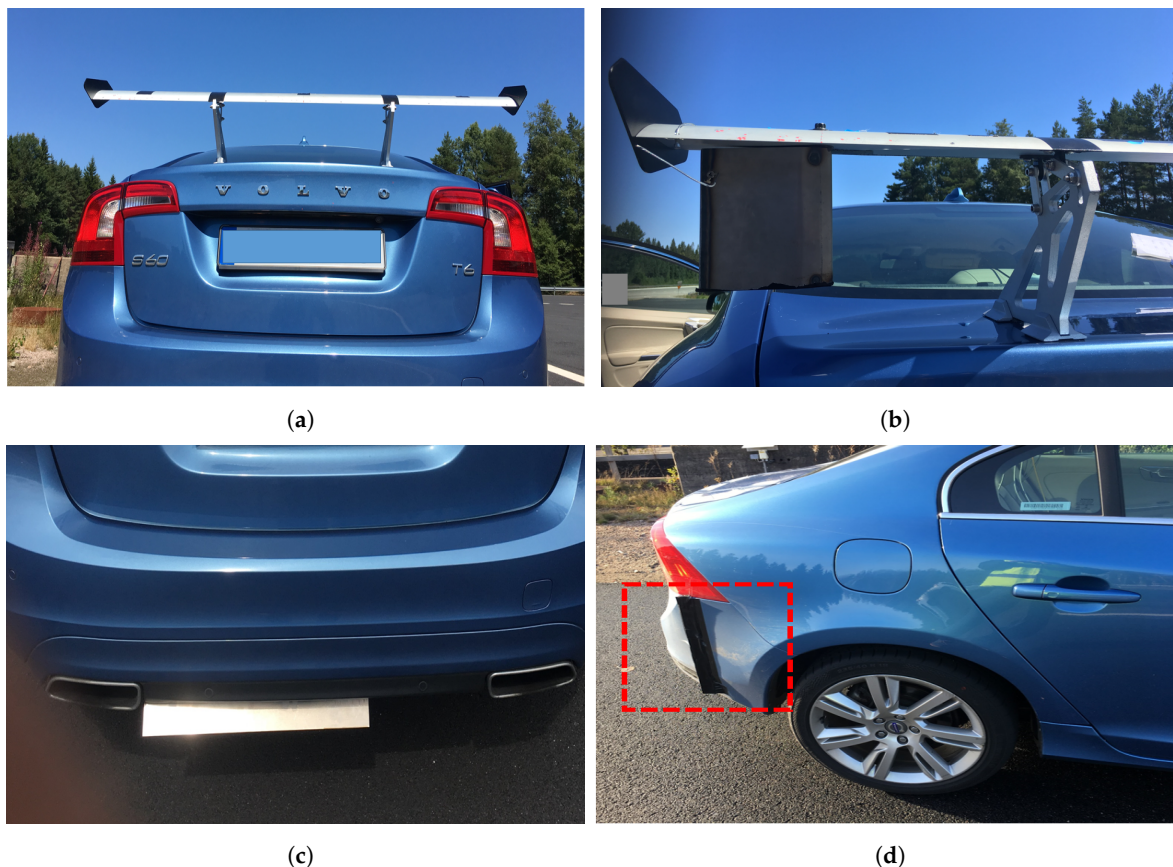
Figure 3. Aerodynamic Devices: (a) Inverted Wing [w]. (b) Inverted Wing with Fin [w-f]. (c) Anti-diffuser [a]. (d) Side-kicks [s].
