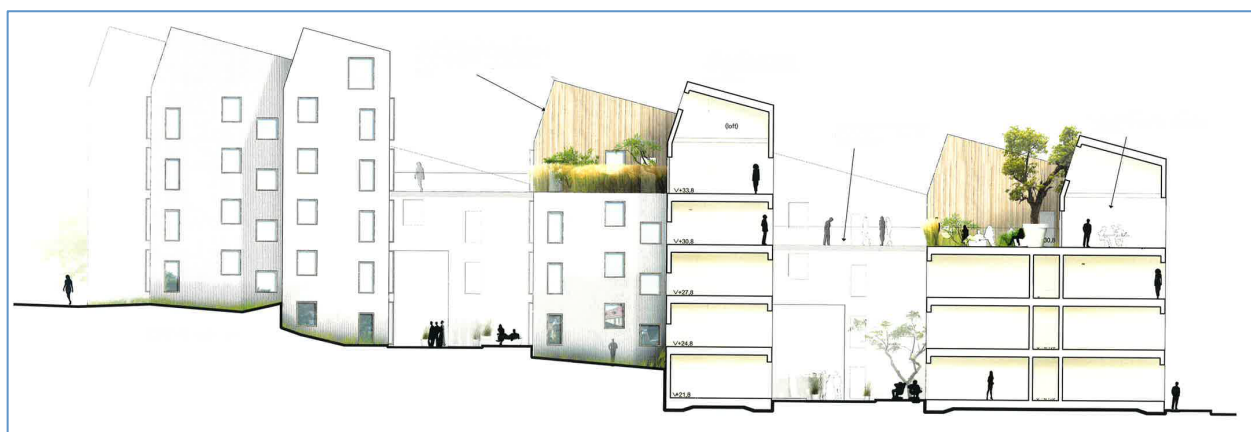
Figure 4. Winning design. Cross section showing the "hubs" on top of the building. Illustration: Lindbäcks bygg AB and White arkitekter 2013.
