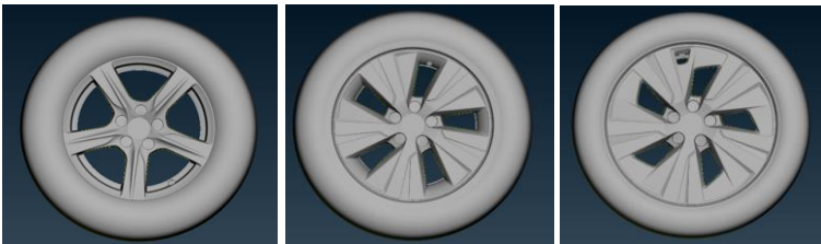
Figure 5. Three rim designs investigated (baseline – left, new designs – middle and right)
