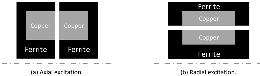
Figure 4-12 Axial and radial excitation.
