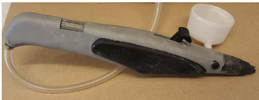
Figure 3. The Aztek A470 Airbrush. The solution is poured in the sample cup and nitrogen was used as the carrier gas. The nozzle used and shown on the picture is a 0.30 mm general purpose nozzle and several types of nozzles are available.
