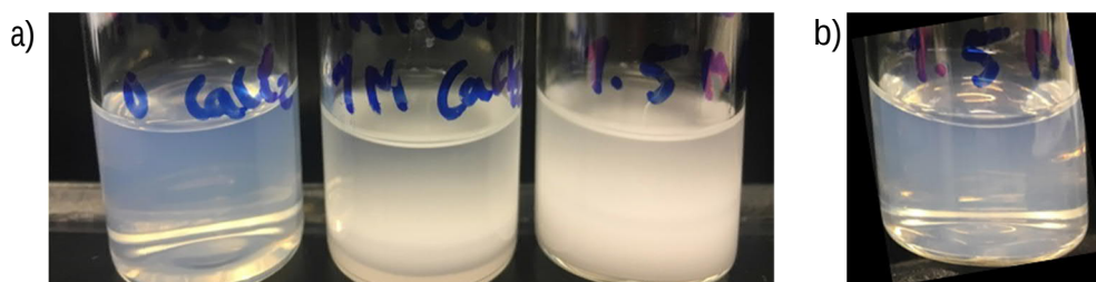
Figure 28. a) Diluted suspensions of mPEG 0.74 -SiNP with no added salt, with 1 M \text{CaCl}_2 and with 1.5 M \text{CaCl}_2 , from left to right, at 3.5 wt% of \text{SiO}_2 . The samples have been heated to 110 °C and clouding was observed for the two samples containing \text{CaCl}_2 . b) Shows the sample with 1.5 M \text{CaCl}_2 cooled to room temperature, and the original turbidity was regained.
