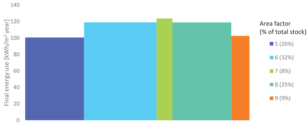
Fig. 4. Final energy use of buildings in the stock aggregated to value factor for the value area corresponding to each building. The width represents the share of heated floor area of buildings per area factor in relation to the entire portfolio [%]. The value factor has been rounded down to the nearest integer.
