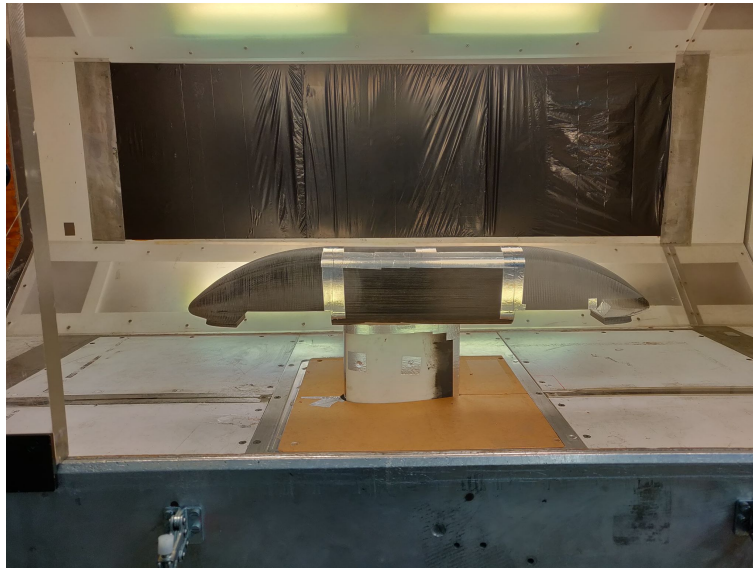
Figure 3: Placement of the model on the support inside of the wind tunnel. (Ground clearance not adjusted.)
