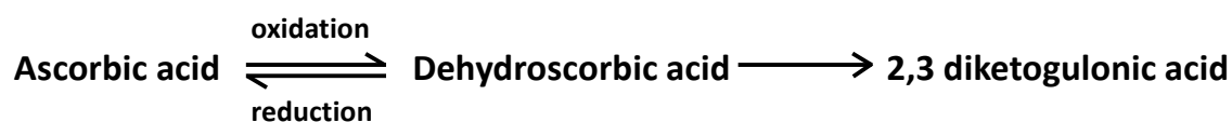
Figure 4: The oxidation of ascorbic acid to dehydroascorbic acid and further to 2,3 diketogulonic acid.
