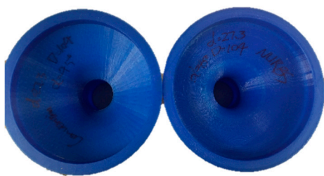
Figure 4. Printed cones (the right cone is the NURBS cone). The shapes are depicted in Figure 3.
