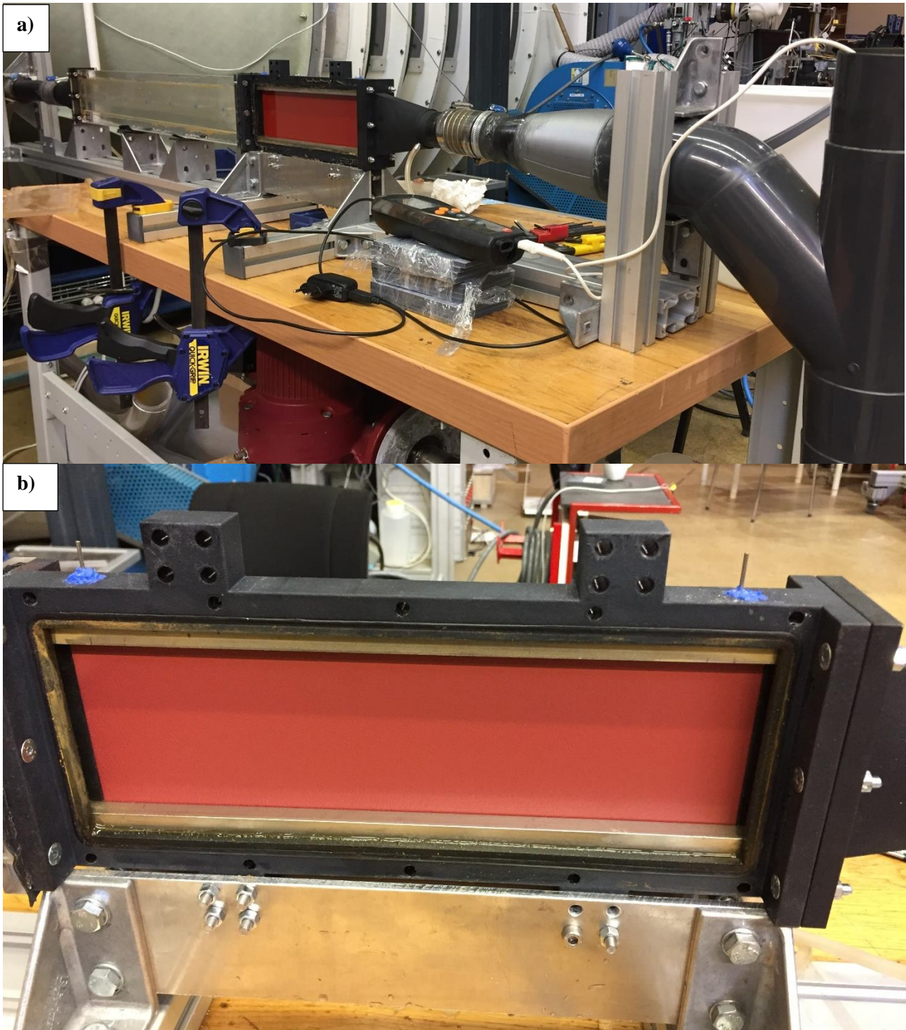
Figure 1. a) The flowcell overview; b) Installation of coated test panel (red) in the testing section
