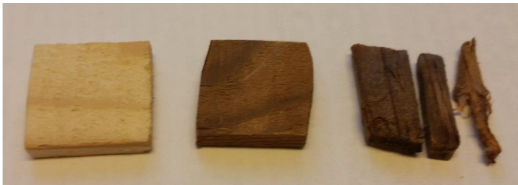
Fig. 3.3 From left to right: Native, SEW, and SEIW. Notice the color change after treatment present in both samples subjected to steam explosion. The SEIW samples show distinct ruptures mostly in the fiber direction.
