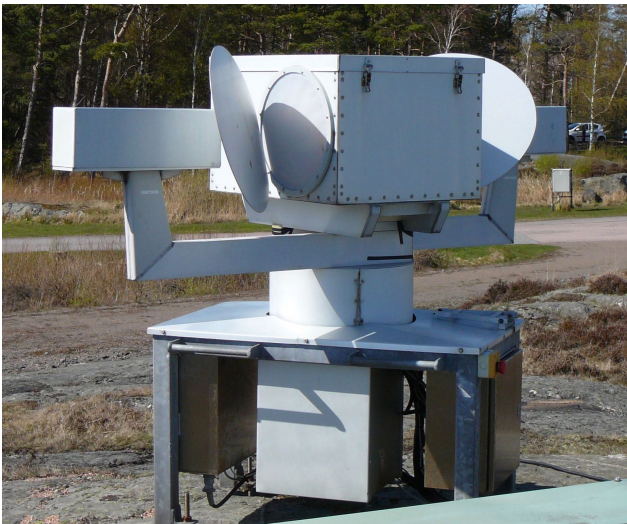
Figure 4. The water vapour radiometer (WVR) Konrad at the Onsala Space Observatory.
