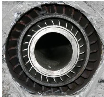
Figure 6. Photograph of the burner used in the LKAB KK2 plant. Solid fuel and transport air are injected through the central pipe, and swirl air through the inner swirl register. The outer swirl register is not in use.
